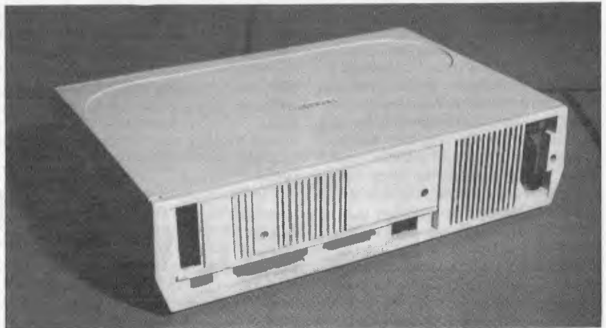
Pop out panels at the back allow sockets for add-on interface cards.
